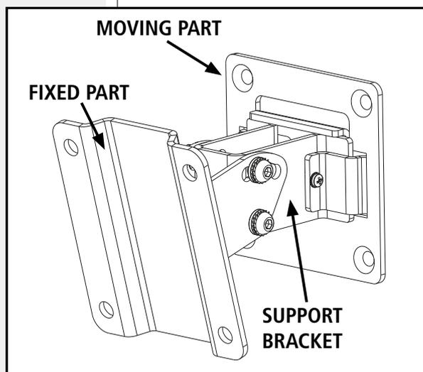
The MOVING PART of the accessory must be fixed directly on the back of the speaker with 4 M6 flat head screws (already placed on the speaker). On the COMPACT M 08 model the accessory can be fixed in two different positions (as shown in the picture below).
