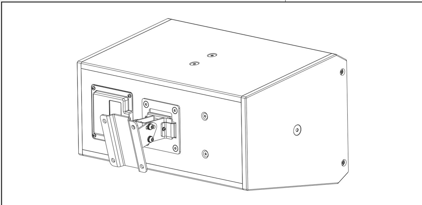
3. Then, place the speakers on the support braket and tighten the two lateral bolts.
