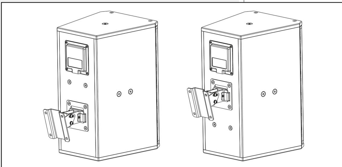
It is also possible the loudspeaker horizontal mounting (see the figure below).
